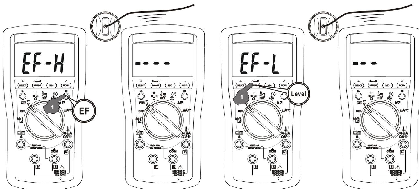
● **Non-Contact EF-Detection:** An antenna is located along the top-left end of the meter, which detects electric field surrounding energized live conductors. It is ideal for tracing live wiring connections, locating wiring breakages and to distinguish between live and earth connections.
